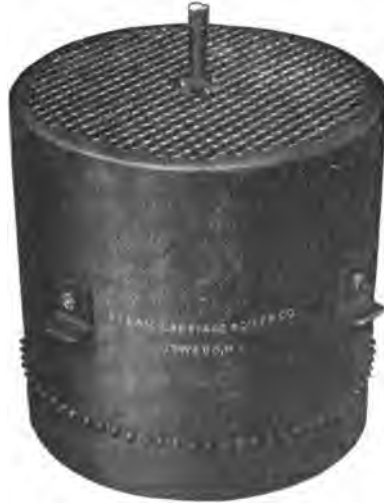
FIG. 145.—Small Carriage Boiler made from a seamless steel pressing, the lower tube plate being flanged over and riveted in, as indicated at the base of the figure, this being the only seam in the structure.
